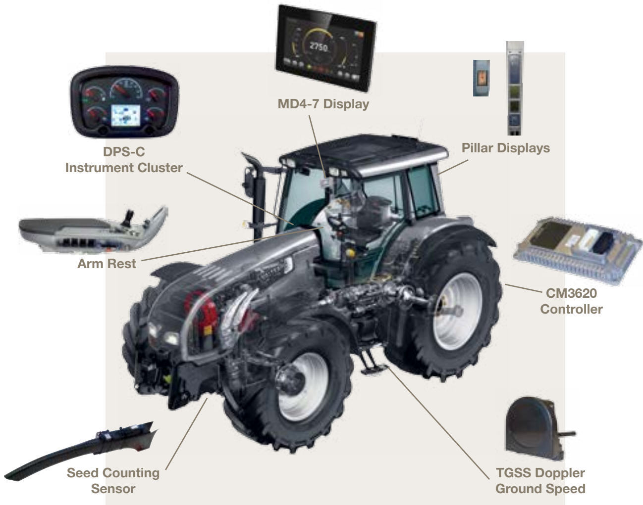
Illustration shows possible product applications in an agricultural tractor. -image courtesy of Valtra Inc.
