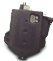
CFM56 engine reservoir
