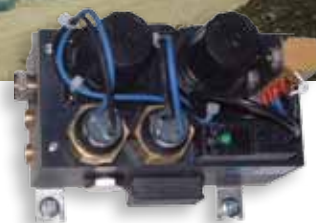
Fully automatic lift/lower controls preventing vehicle overload
